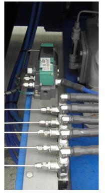
The suffix indicates how many traps the system will drain, for instance the MK-4-5 will drain all five traps of a five stage compressor such as Stark 100, 80, and 55 CFM compressors
